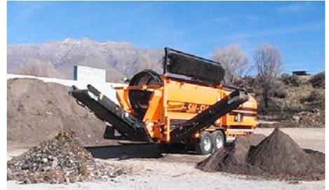
**Rotating screen separates dirt and trash.**
