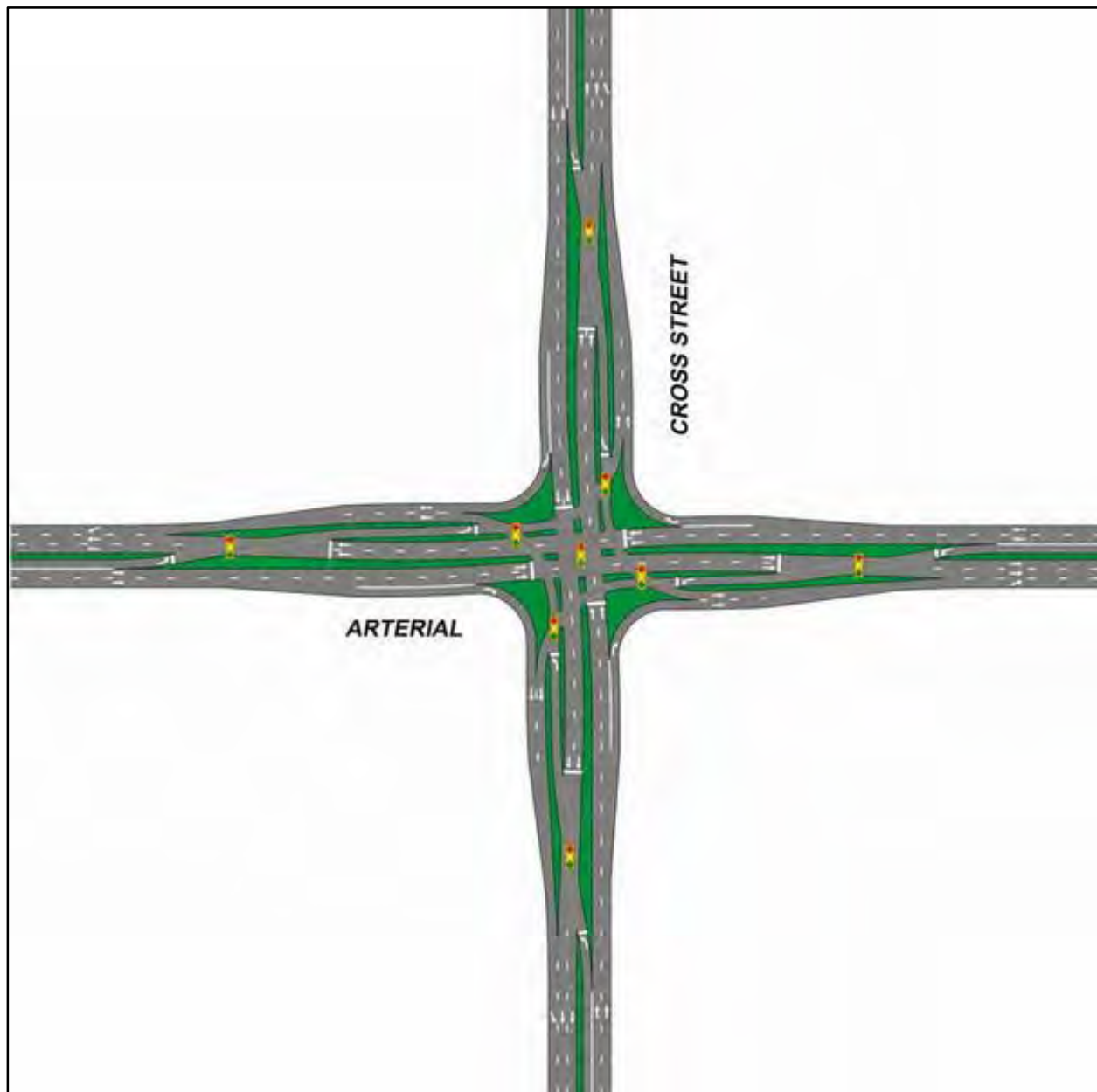
Figure 28: Continuous Flow Intersection (CFI) Example
