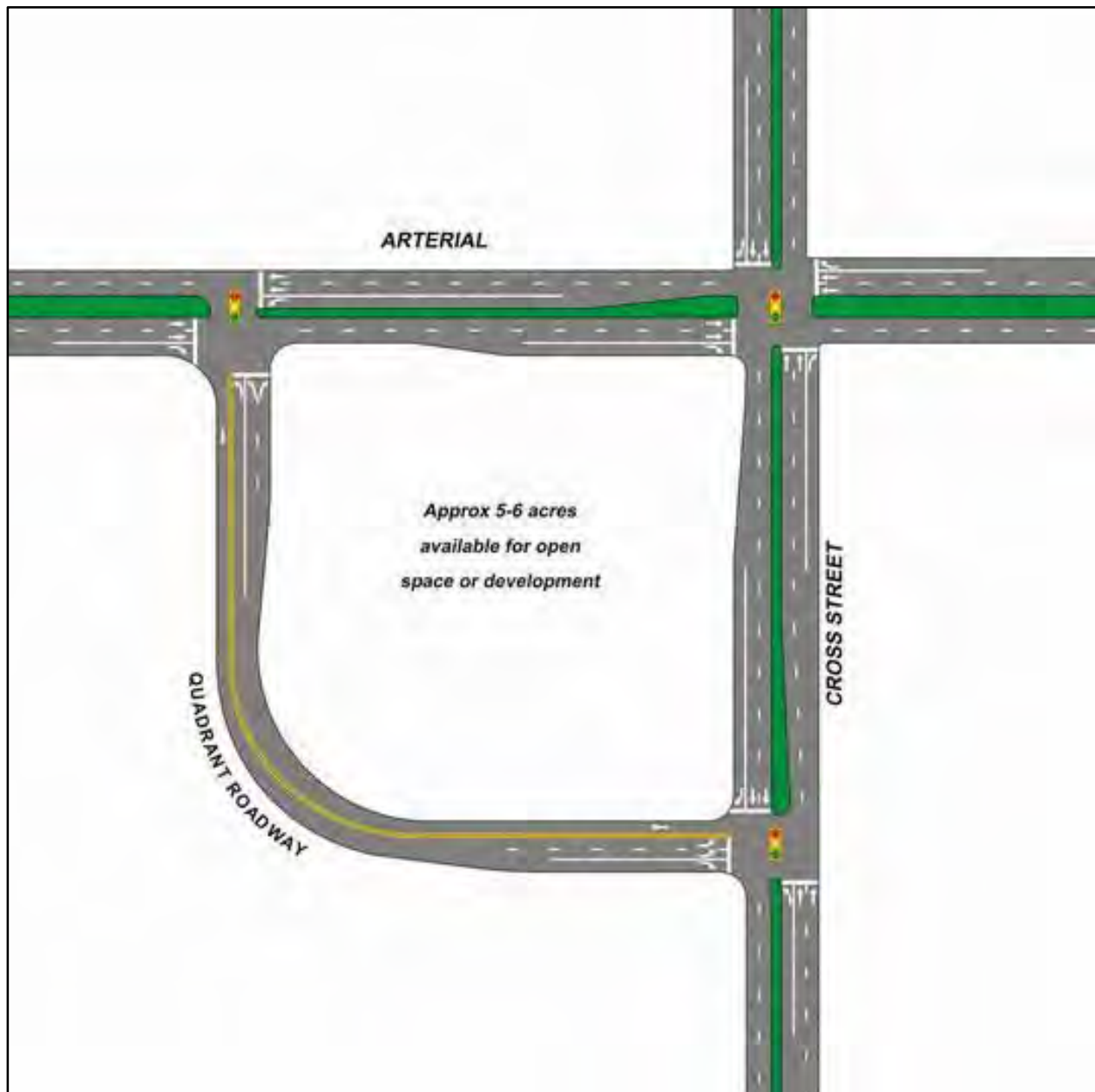
Figure 30: Quadrant Roadway Example
