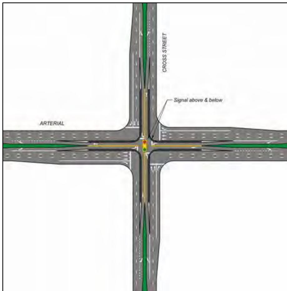
Figure 27: Center Turn Overpass (CTO) Example
